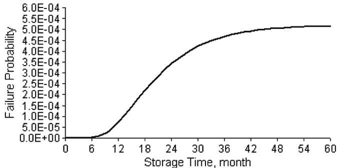
Fig. 8. Failure probability plot in terms of tin whiskers caused leads bridging.
