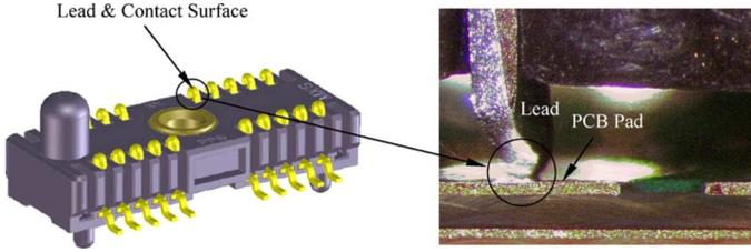
Fig. 1. Sketch of a compressive contact connector.
