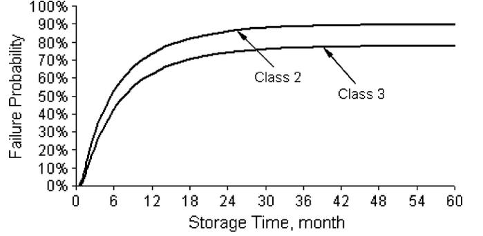
Fig. 7. Failure probability plots in terms of NEMI acceptance criteria.
