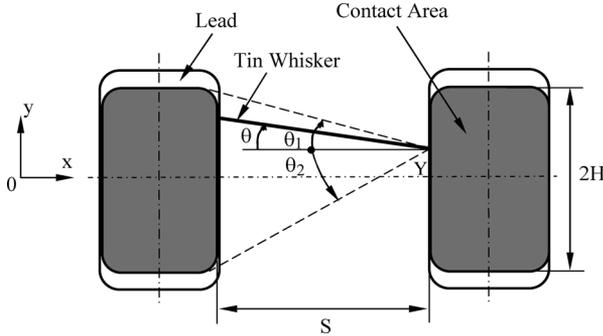
Fig. 2. Schematic showing a tin whisker bridging two adjacent leads.
