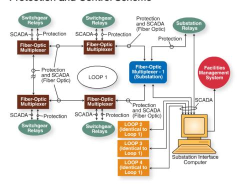
The new infrastructure features a closed-loop primary-voltage distribution automation system, where switchgear and relays communicate through a multiplexed fiber-optic network.
