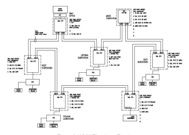
Figure 2, WMU Fiber Loop Topology
